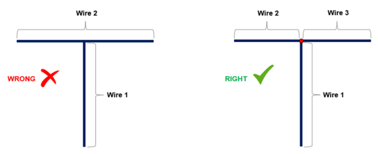
Fig. 1: Incorrect and correct methods for connecting wires.
